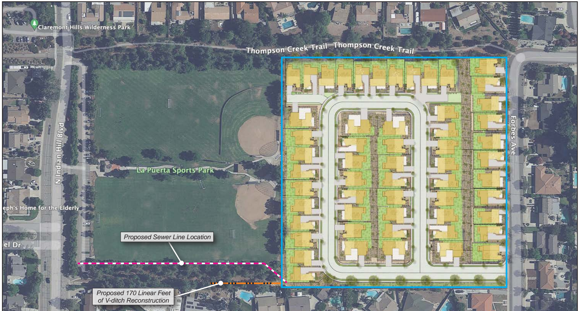
Figure 3-10 - Proposed Offsite Sewer and Drainage Improvements
