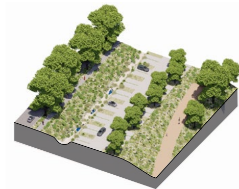
BIOSWALE NEAR PARKING
