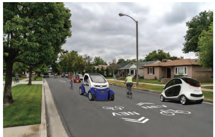
Neighborhood electric vehicles (NEVs) are a lower-impact alternative to standard cars for a carshare program. NEVs, however, are restricted to travel on certain types of streets. Above, a rendering of an NEV-friendly bicycle boulevard.
