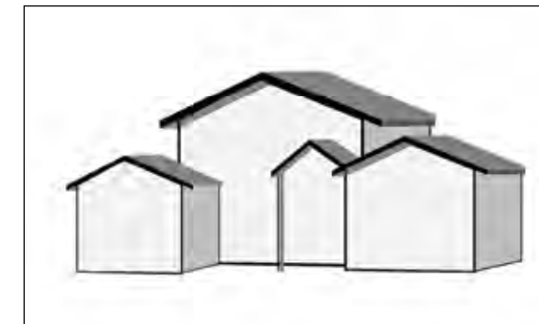
Second story additions with roof forms and slopes that match those of the original structure are most compatible
