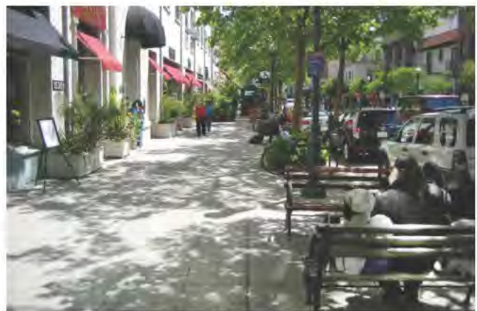
Frontages in a commercial environment with clearly articulated pedestrian, landscape/furniture, and curbside flex zones.
