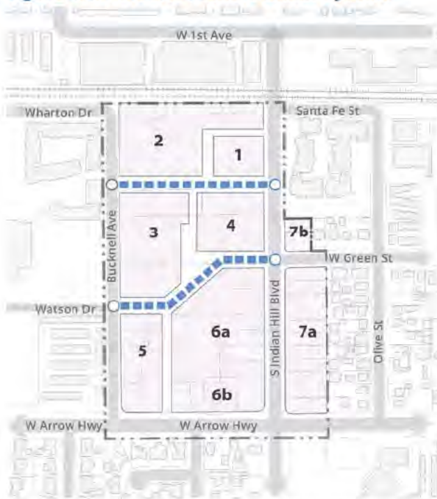
Figure 4.4.C On-site Potable Water System
