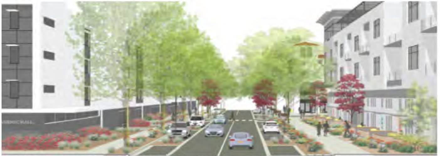
Bucknell Avenue Proposed Bioswale (See also Section 3.12.D.4): A continuous landscape bioswale is proposed along the east side of Bucknell Avenue, with parking lane planters proposed on both sides of the street. Together, these retrofits could provide significant retention and infiltration of stormwater runoff by simply repurposing Bucknell Avenue's excess street width.
